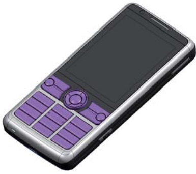
Model for Drop Test Simulation By courtesy of Sony Ericsson Mobile Communications AB
