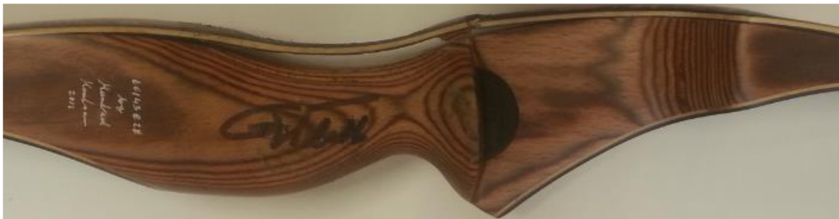
Fig.3: Delamination failure in the bow grip between the wood handle and the lamellar structure of the limbs
