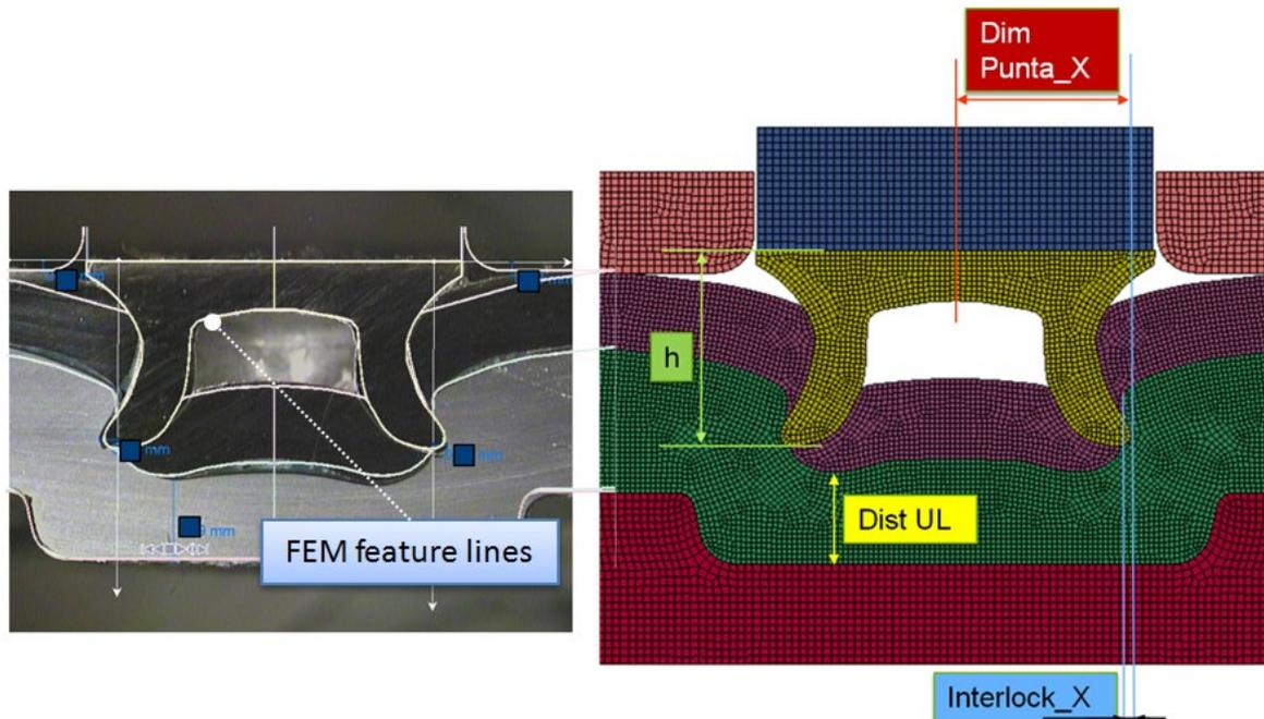
Fig.3: Overlapped image - Experimental vs. Numerical
