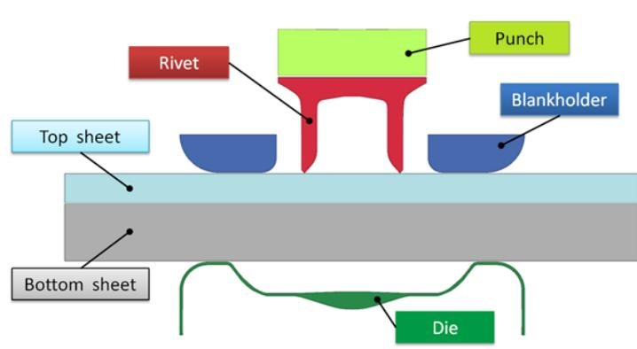
Fig. 1: SPR tool setup.
