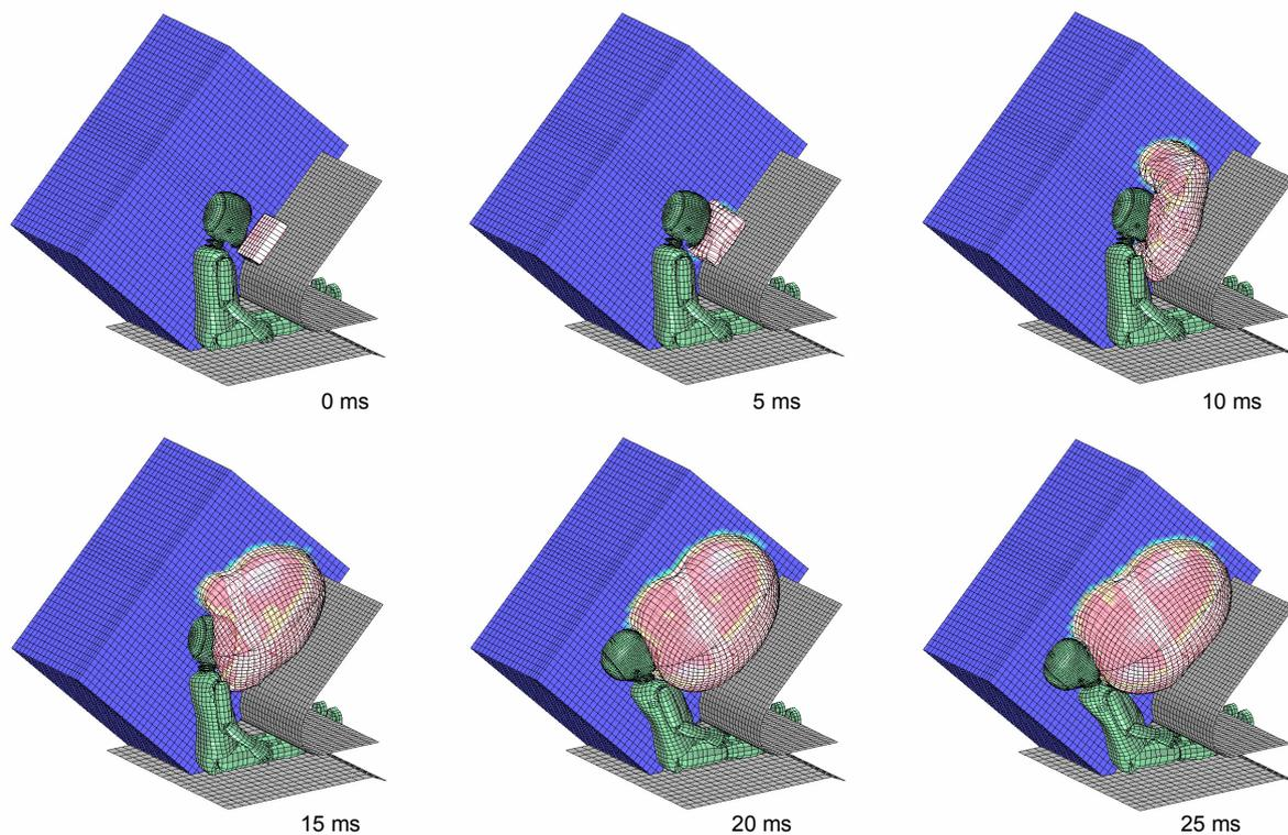
*Figure 9: Unfolding of OoP-airbag problem with Euler-method (Euler-mesh cut open)*
