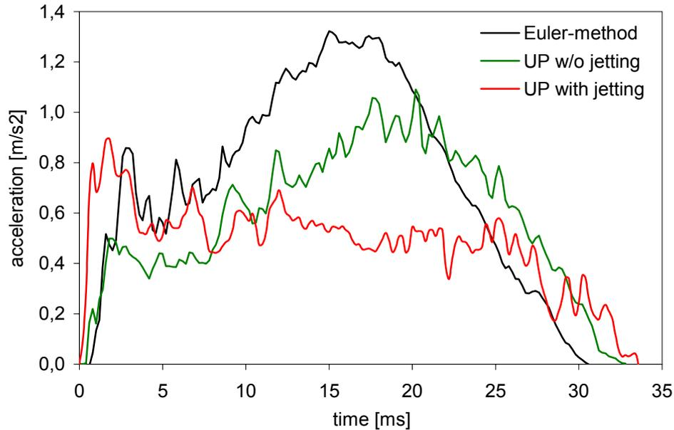
Figure 8: Acceleration of steel pipe in z-direction with different modelling techniques
