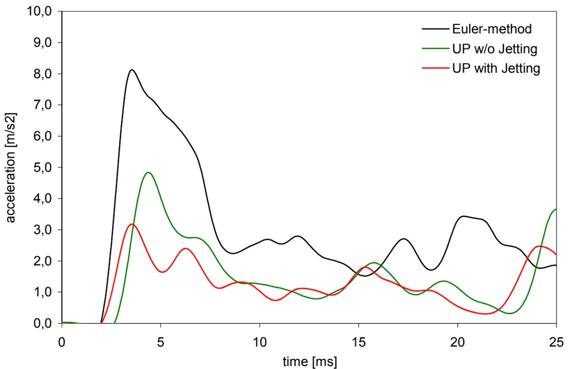
Figure 11: Total acceleration of thorax with different modeling techniques
