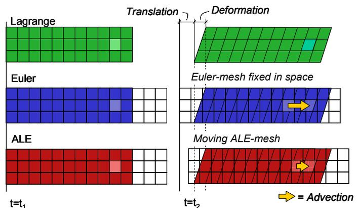
Figure 4: Comparison of Lagrange, Euler and ALE-description
