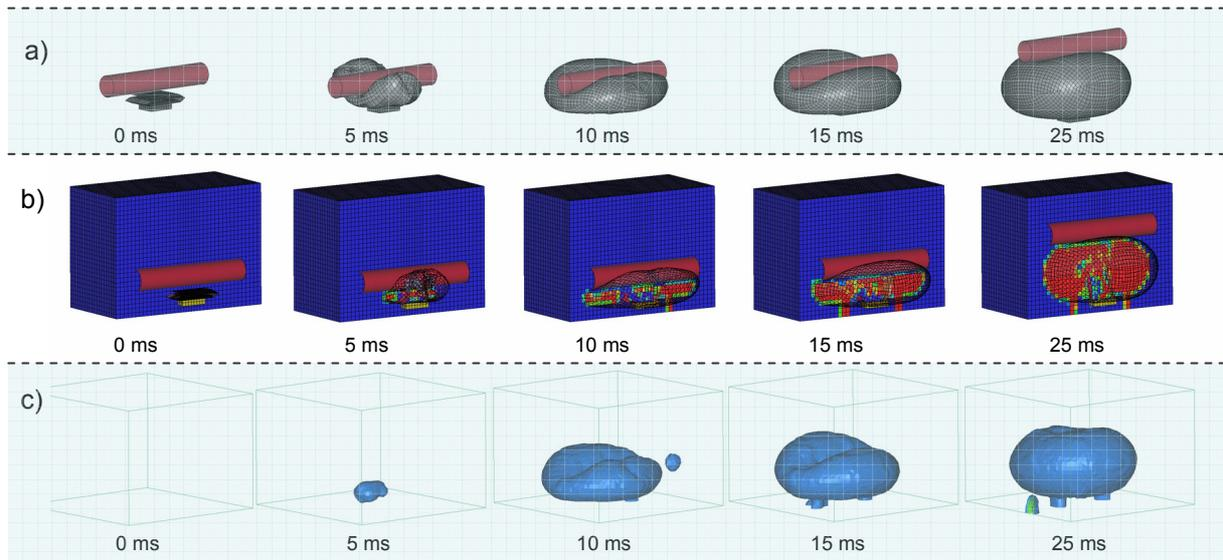
Figure 7: Unfolding of airbag: a) Control-Volume b) Euler-method and c) iso-surface of inflowing gas
