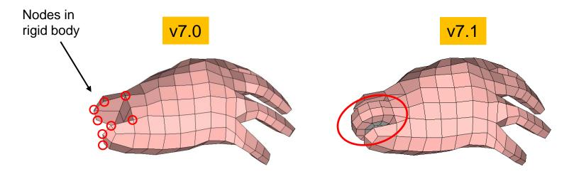
This change is expected to eliminate erroneous signal spikes as the wrist impacts the car interior.
