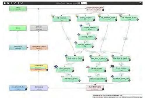
Figure 1: Flowchart-based GUI of LS-OPT® Version 5. The interconnected stages between Sampling and Metamodels represent the flow of multidisciplinary solution stages.
