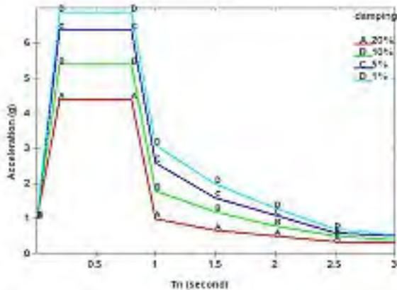
Figure 7. Input spectra for different damping
