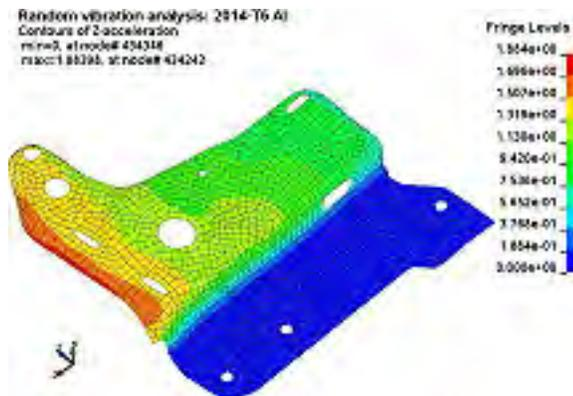
Figure 5. RMS of Z-acceleration
