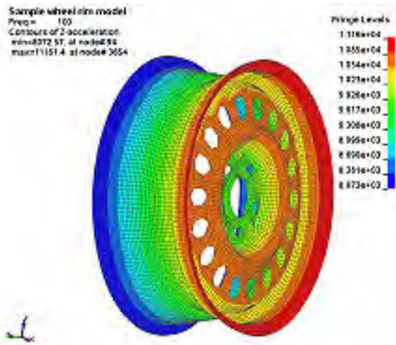
Figure 3. Z-acceleration at frequency 100 Hz
