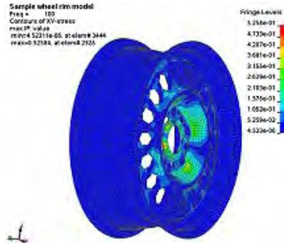
Figure 4. xy shear stress at frequency 100 Hz
