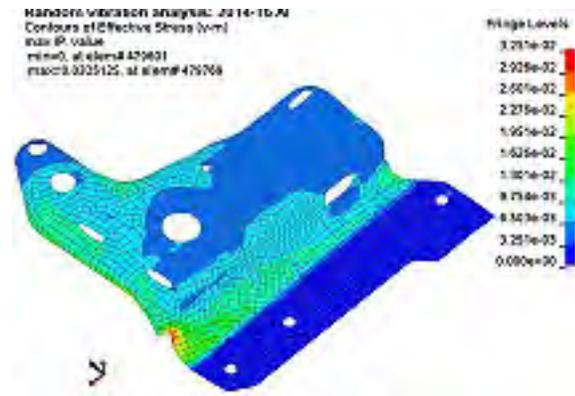
Figure 6. RMS of Von Mises stress
