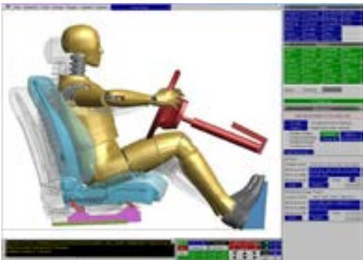
There are a number of functions available within Oasys PRIMER to aid with setting up and positioning occupant dummies within a model. These include:
