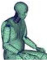
The BioRID 2 model is used for the investigation of seat performance under rear impact loads, with the focus on the prediction of whiplash injuries. It is developed by DYNAmore.
