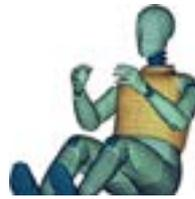
FTSS develops validated dummy models based on their physical anthropomorphic test devices (ATD), that are used in car crash testing all over the world.
